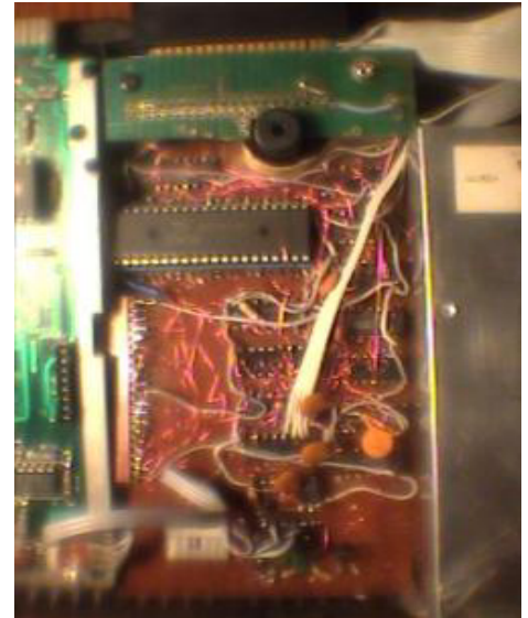
THE FLOPPY DISK CONTROLLER BOARD. IT SITS BETWEEN THE MAIN CPC BOARD AND THE 3.5 INCH DISK DRIVE.
