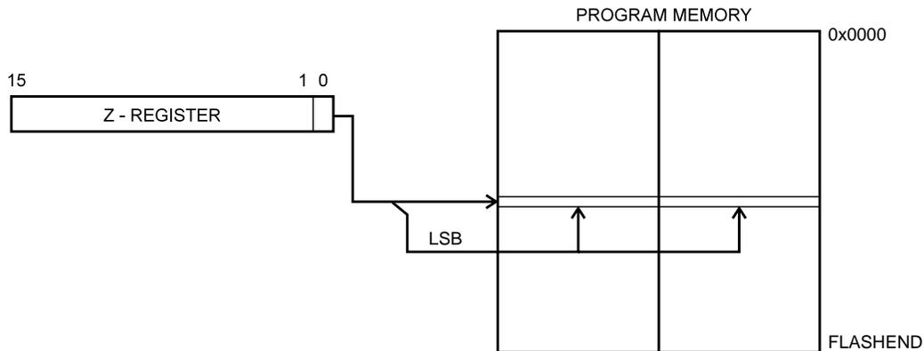
Constant byte address is specified by the Z-register contents. The 15 MSBs select word address. For LPM, the LSB selects low byte if cleared (LSB = 0) or high byte if set (LSB = 1). For SPM, the LSB should be cleared. If ELPM is used, the RAMPZ Register is used to extend the Z-register.
