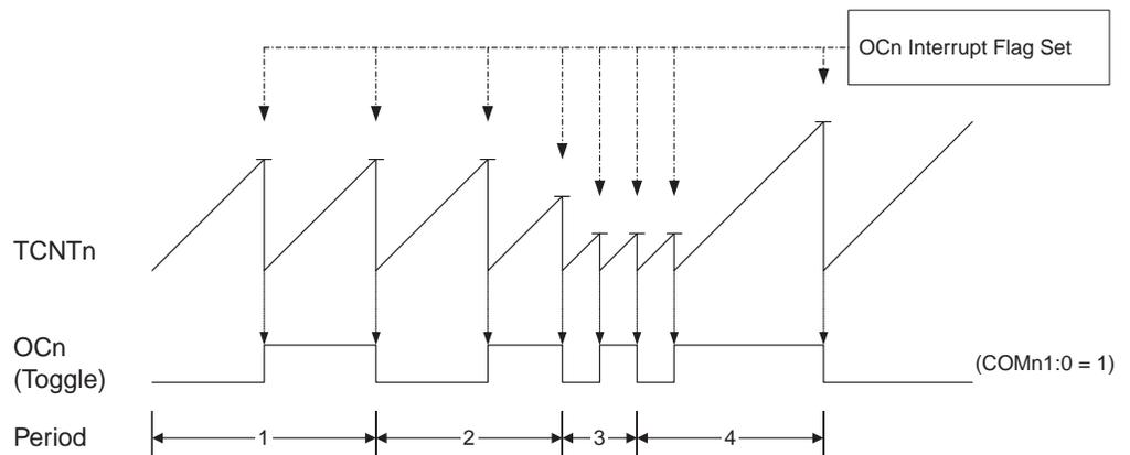
An interrupt can be generated each time the counter value reaches the TOP value by using the OCF0 Flag. If the interrupt is enabled, the interrupt handler routine can be used for updating the TOP value. However, changing TOP to a value close to BOTTOM
