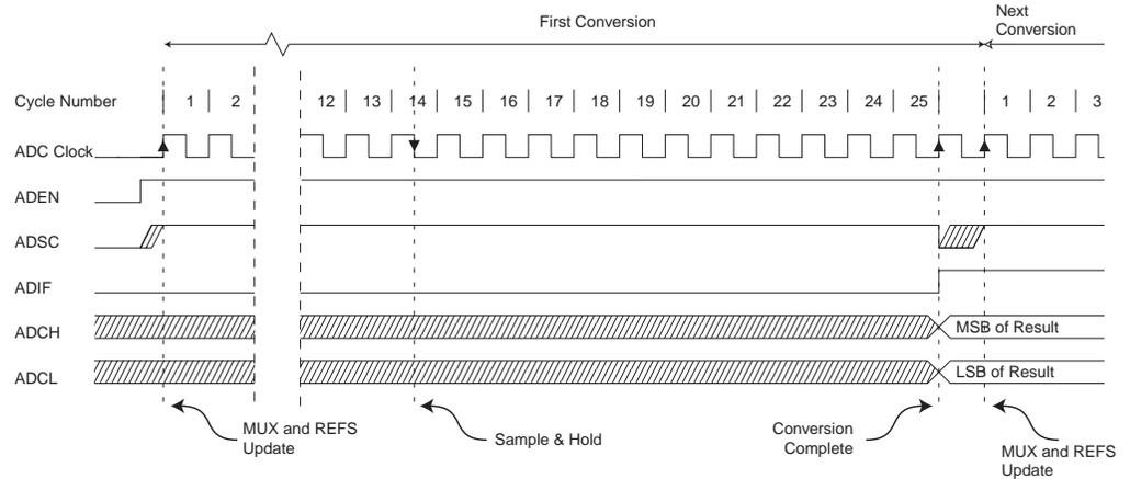
**Figure 102. ADC Timing Diagram, Single Conversion**
