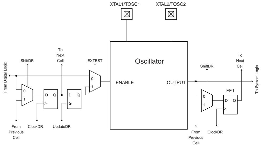
Table 90 summarizes the scan registers for the external clock pin XTAL1, Oscillators with XTAL1/XTAL2 connections as well as 32 kHz Timer Oscillator.
