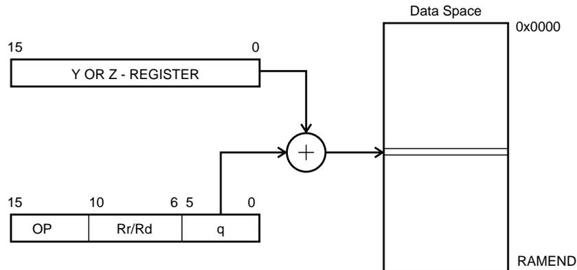
Operand address is the result of the Y- or Z-register contents added to the address contained in 6 bits of the instruction word. Rd/Rr specify the destination or source register.
