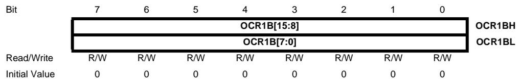
The Output Compare Registers contain a 16-bit value that is continuously compared with the counter value (TCNT1). A match can be used to generate an output compare interrupt, or to generate a waveform output on the OC1x pin.
