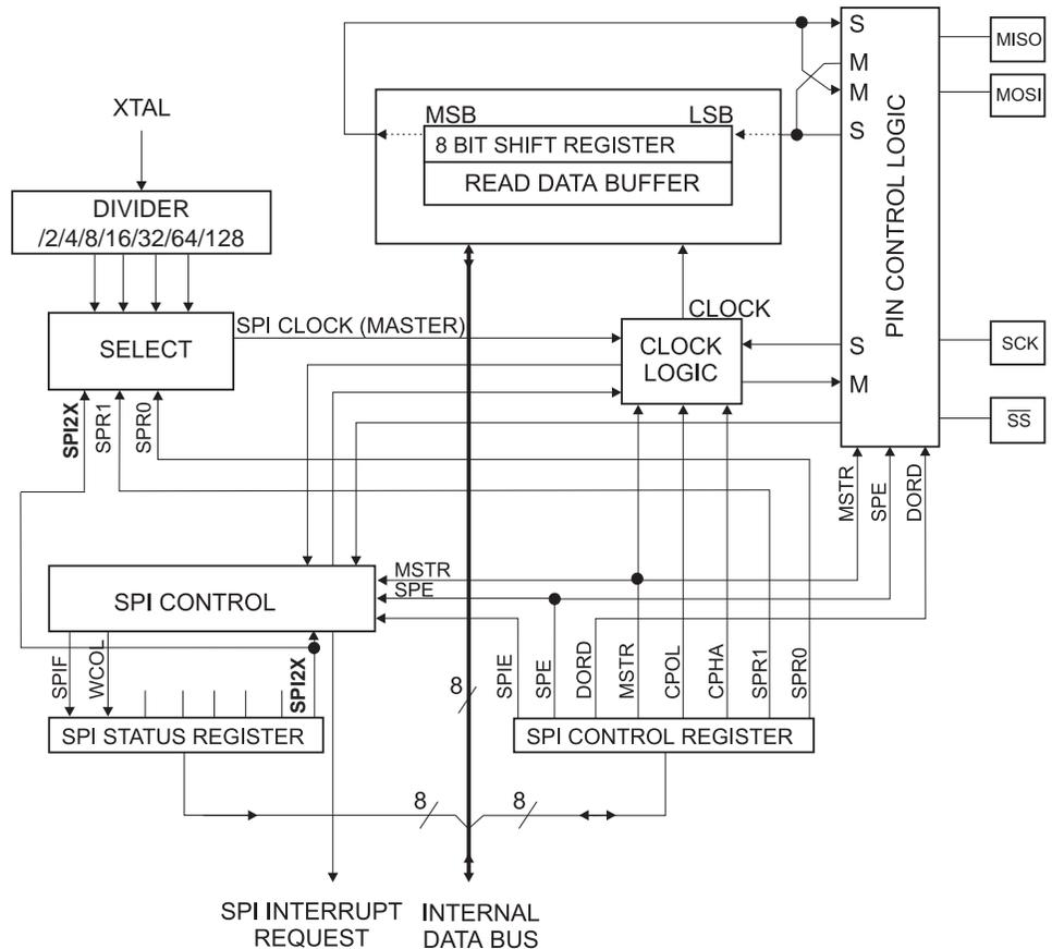
Note: 1. Refer to Figure 1 on page 2, and Table 25 on page 56 for SPI pin placement.
