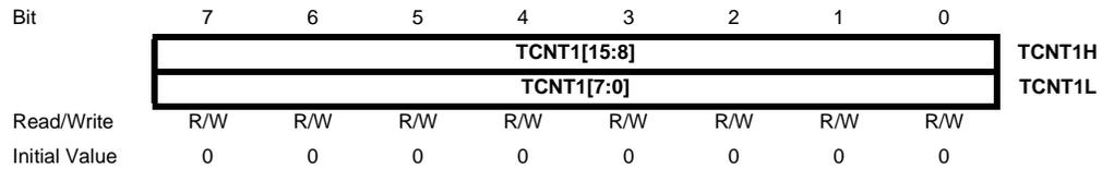
The two *Timer/Counter I/O* locations (TCNT1H and TCNT1L, combined TCNT1) give direct access, both for read and for write operations, to the Timer/Counter unit 16-bit counter. To ensure that both the high and Low bytes are read and written simultaneously when the CPU accesses these registers, the access is performed using an 8-bit temporary High Byte Register (TEMP). This temporary register is shared by all the other 16-bit registers. See “Accessing 16-bit Registers” on page 89.
