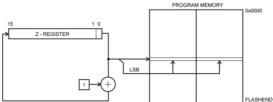
Constant byte address is specified by the Z-register contents. The 15 MSBs select word address. The LSB selects low byte if cleared (LSB = 0) or high byte if set (LSB = 1). If ELPM Z+ is used, the RAMPZ Register is used to extend the Z-register.
