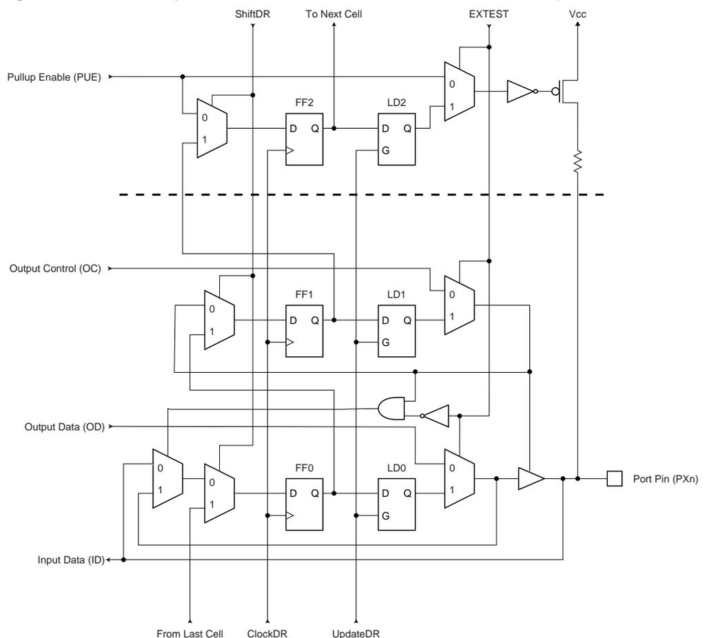
**Figure 117. General Port Pin Schematic Diagram<sup>(1)</sup>**
