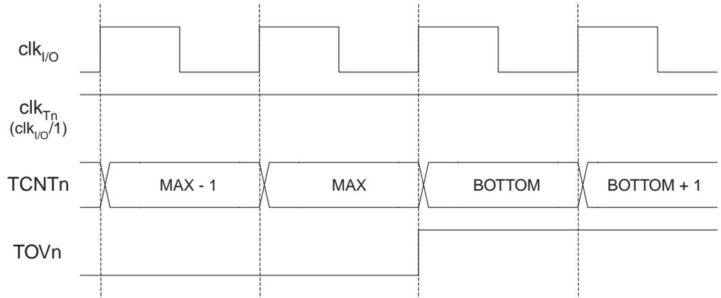
Figure 35 shows the same timing data, but with the prescaler enabled.
