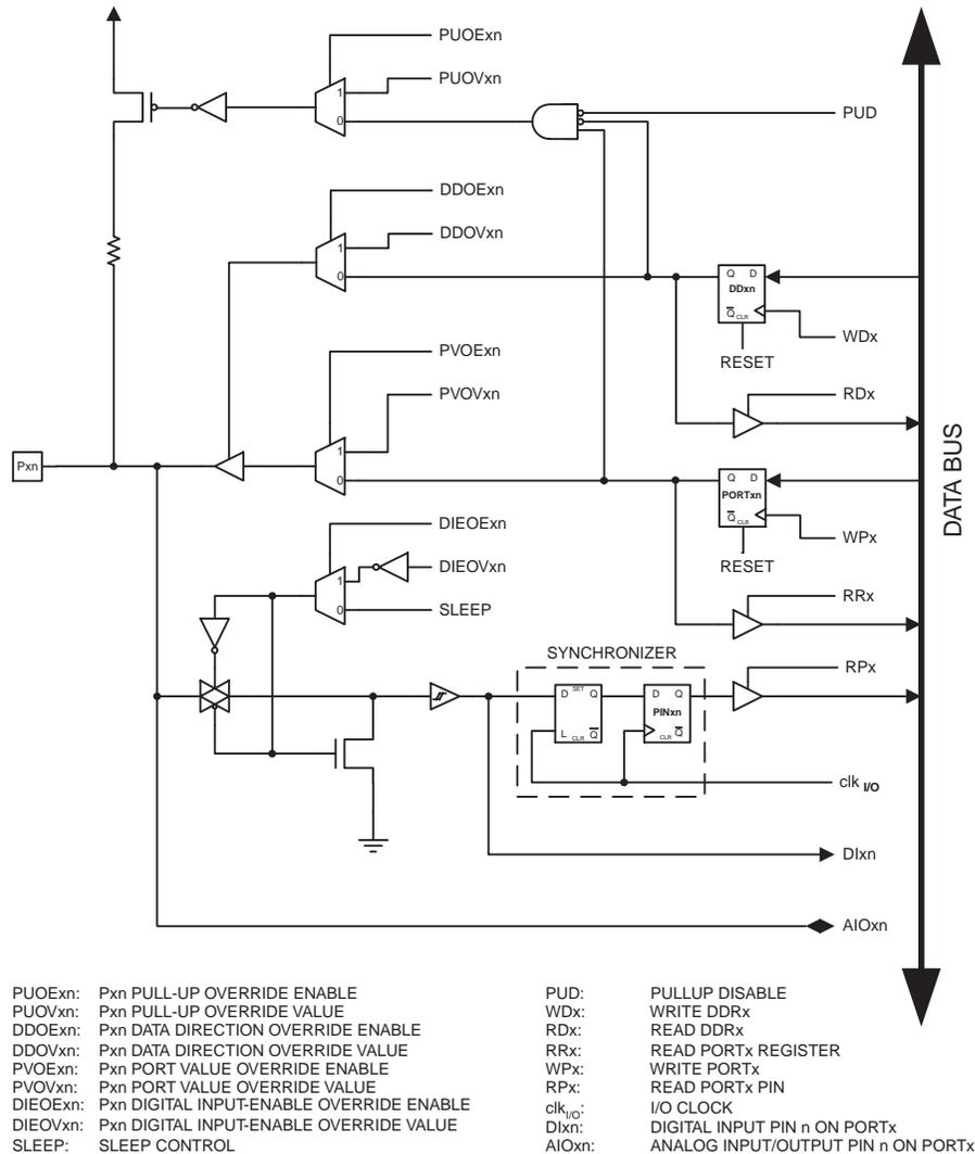
Note: 1.  $WP_{xn}$ ,  $WD_{xn}$ ,  $RR_{xn}$ ,  $RP_{xn}$ , and  $RD_{xn}$  are common to all pins within the same port.  $clk_{I/O}$ ,  $SLEEP$ , and  $PUD$  are common to all ports. All other signals are unique for each pin.
